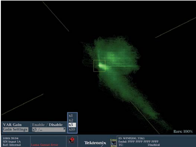
Figure 7. Tektronix waveform monitors can easily and quickly display zoomed, gained or magnified images of various waveform displays, like this 5x zoom of a vectorscope.
