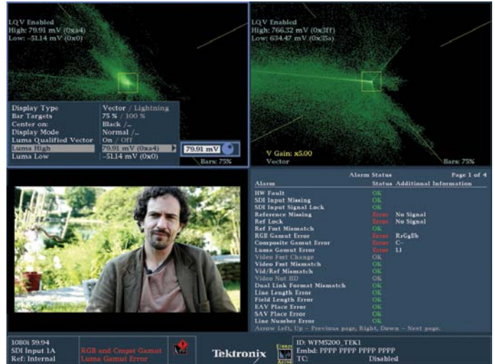
Figure 12. This shows the customization menu for setting the tonal range that the LQV will display. In this case, the LQV will show shadows from below 0mV up through 79.91 mV.
