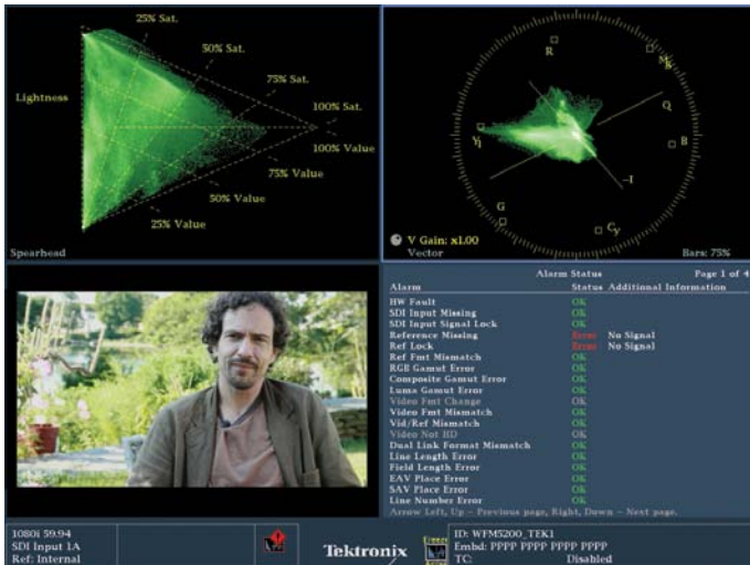
Figure 9. Spearhead and Vectorscope are great complementary displays.
