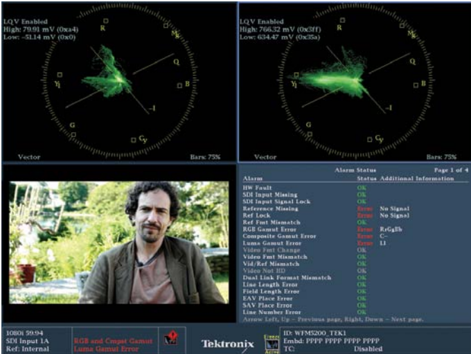
Figure 11. The LQV on the left is showing shadows. The LQV on the right is showing highlights. Notice the blue numerical "High" and "Low" readouts in the upper left corner of each display. This shows the tonal range that each LQV is set to display.
