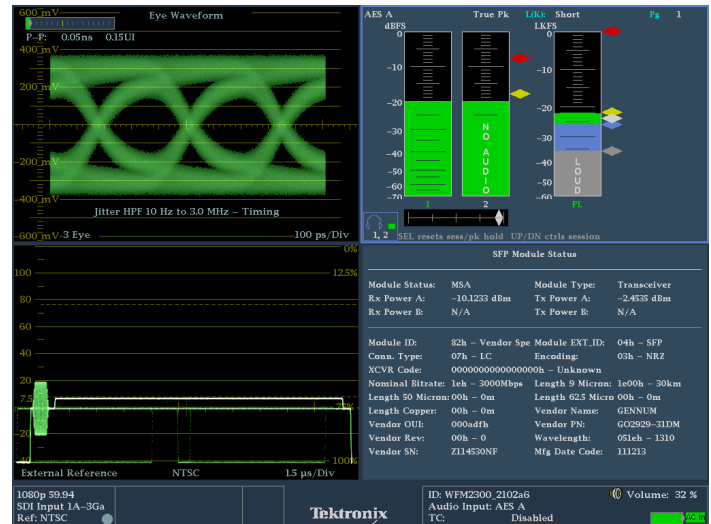
Variety of interface support (Eye display of SDI input, Audio display of AES/EBU input, Waveform display of external reference input, SFP Module Status display of optical input).
