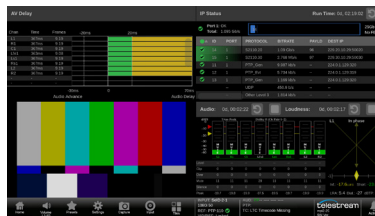
Dolby stream over SDI, ST 2022-6, ST 2110-30/31 will be internally decoded and measured against video. The labeling for each channel is automatically assigned from Dolby metadata.
