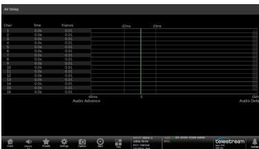
AV Delay measures the time difference of 16 channel audio against video simultaneously. Negative number means audio advance and positive number means audio delay.
