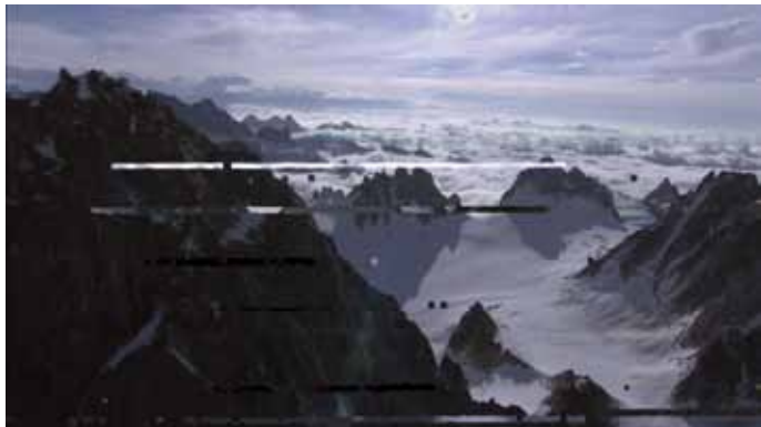
Figure 3.15. Significant loss of RF or IP packets cause blockiness and slice errors.
