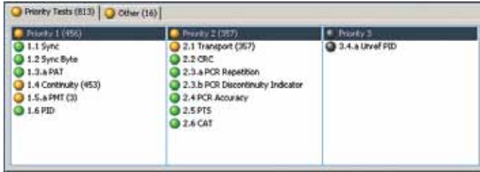
Figure 3.5. TR 101 290 table tabulating several corrupt TS packets as well as lost or missing packets.
