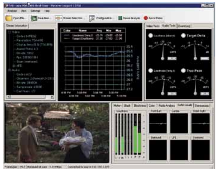
Figure 3.14. Cable broadcast with audio at 2 dB louder than DialNorm. This is a 4 dB increase over the satellite feed.
