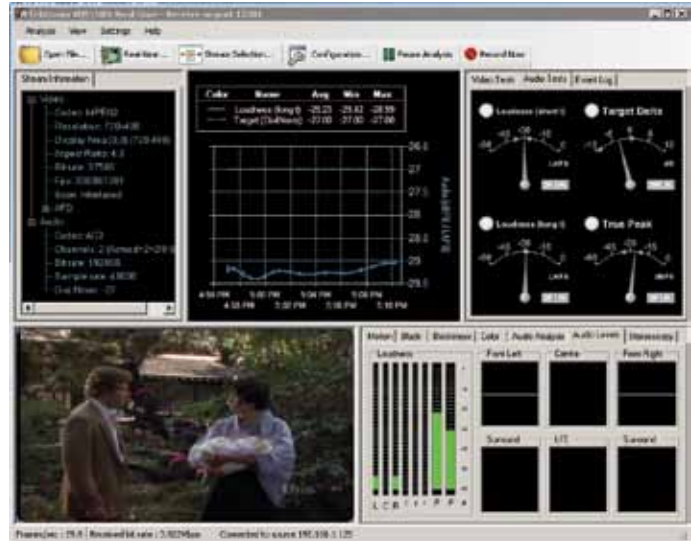
Figure 3.13. Satellite ingest with audio loudness at 2 dB quieter than DialNorm.
