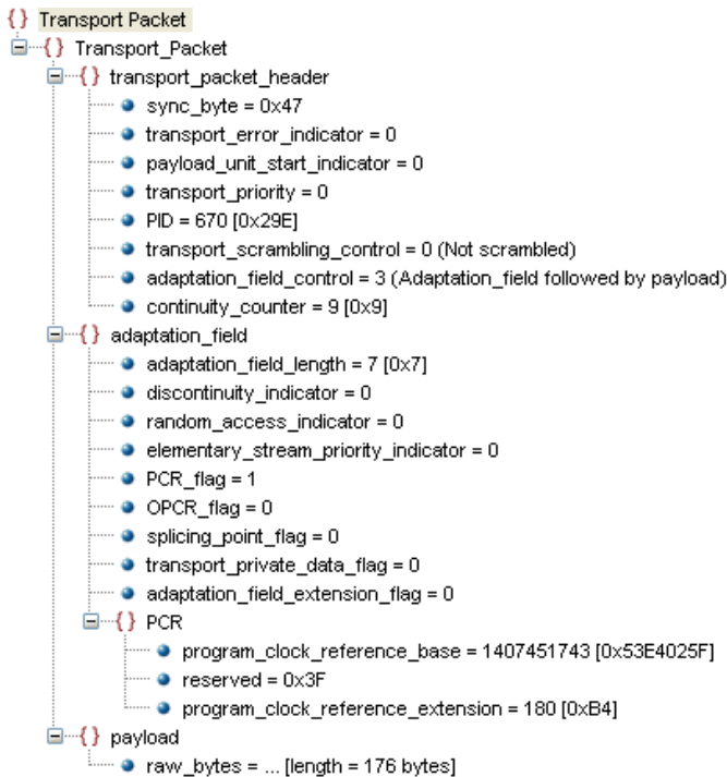
Figure 6-1. ISO/IEC 13818-1 Transport Stream header parameters.
