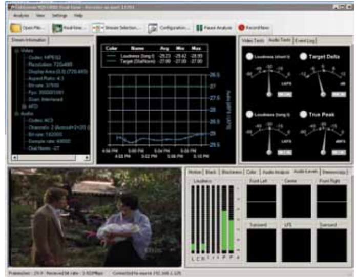
Figure 13-4. Satellite ingest with audio loudness at 2 dB quieter than DialNorm.
