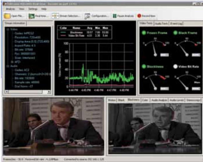
Figure 13-1. Low blockiness from satellite distribution feed.
