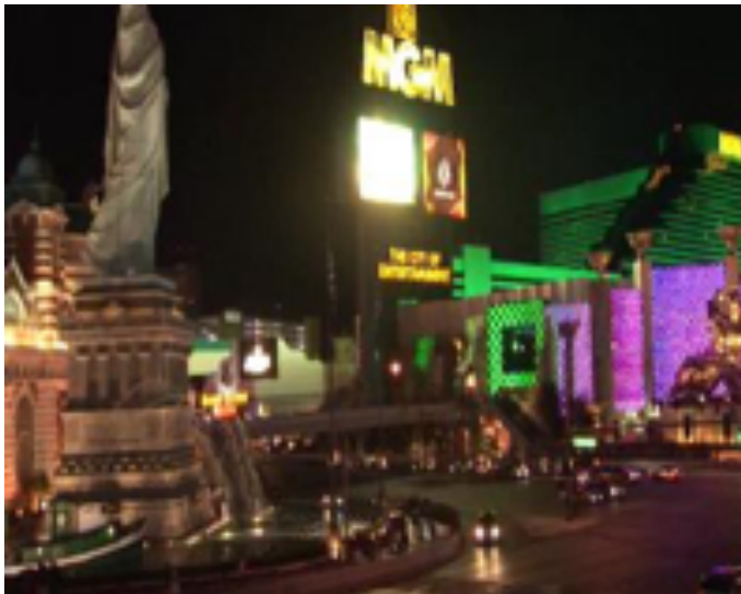
FIGURE 19. “Super white” regions in the image are gamut errors, indicating video levels outside the legal limits for broadcast television.
