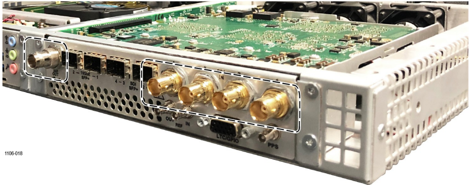
Figure 10: Remove the rear panel plate hardware
