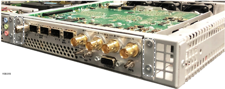
Figure 11: Remove the four rear panel plate screws
