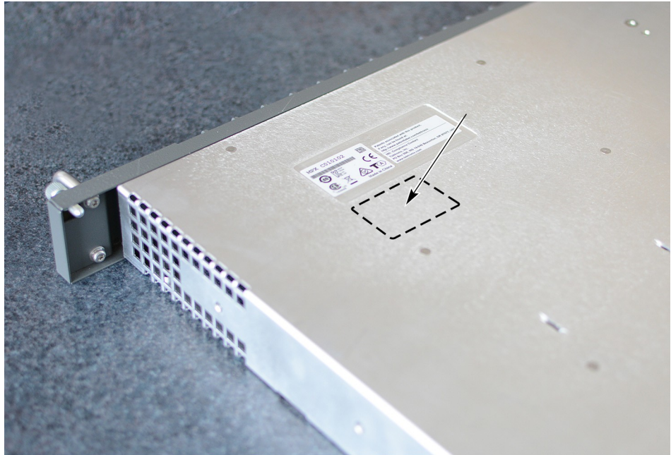
Figure 22: Installing the MPX2-10-UP serial number label
