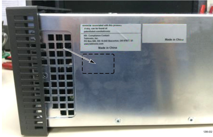
Figure 8: Installing the MPI2-10-UP serial number label
