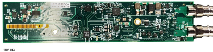
Figure 5: Eye mezzanine board
