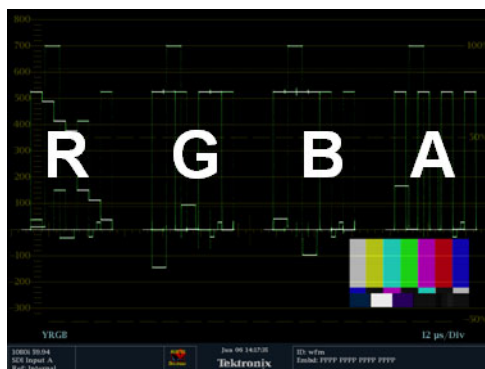
Figure 7: Dual Link information placement in waveform display
