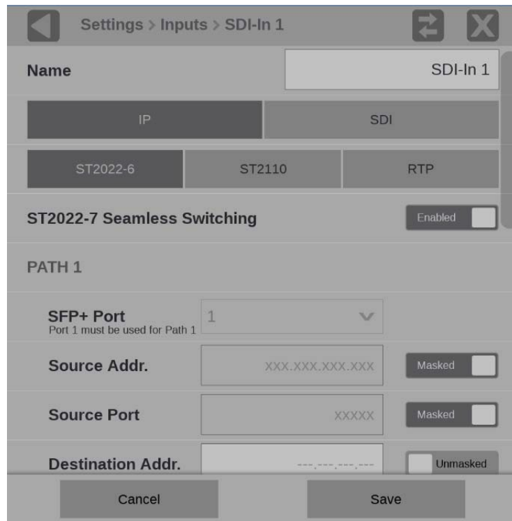
Figure 42: IP input protocols and ST2022-7 seamless switching
