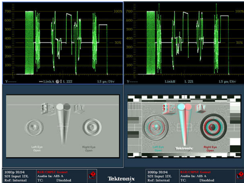
Figure 22: 3D left and right eye images showing a Difference Map and red/cyan anaglyph using SIM
