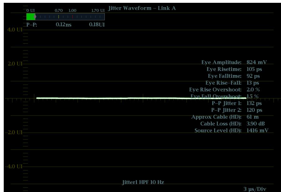
Figure 44: The Jitter display parameters as shown when the instrument is in single-tile mode
