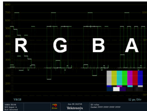
Figure 7: Dual Link information placement in waveform display
