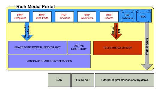
The RMP is integrated with Telestream's FlipFactory via a CSF connector; all digital asset transformation features use the FlipFactory software to convert files from one format to the other.
