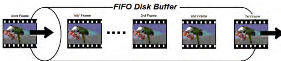
Figure 4–5. FIFO disk buffering enhances file writing performance
