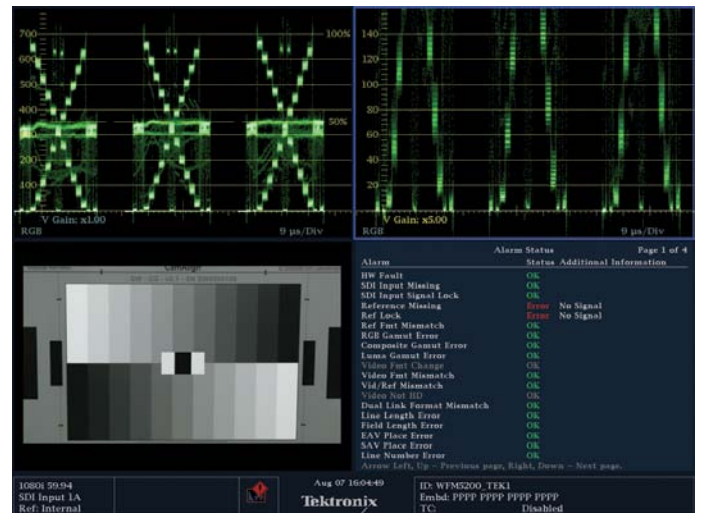
Figure 10. This shows a standard RGB Parade at the top left. On the top right the image is zoomed in and repositioned to show the detail of the shadows.
