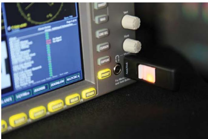
Figure 22. After properly dismounting the "thumb drive" from your computer, plug it in to the USB port on the front of the WFM5200 or other Tektronix waveform monitor.
