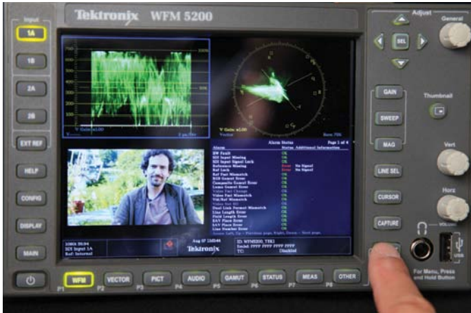
Figure 18. Presets are recalled with two button pushes. Press the reset button (under the finger in this image), then the softkey corresponding to the Preset you want to enable along the bottom of the waveform monitor.
