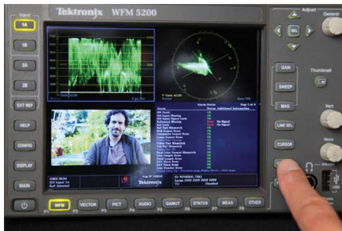
Figure 23. Hold down the preset button, just to the left of the USB port.
