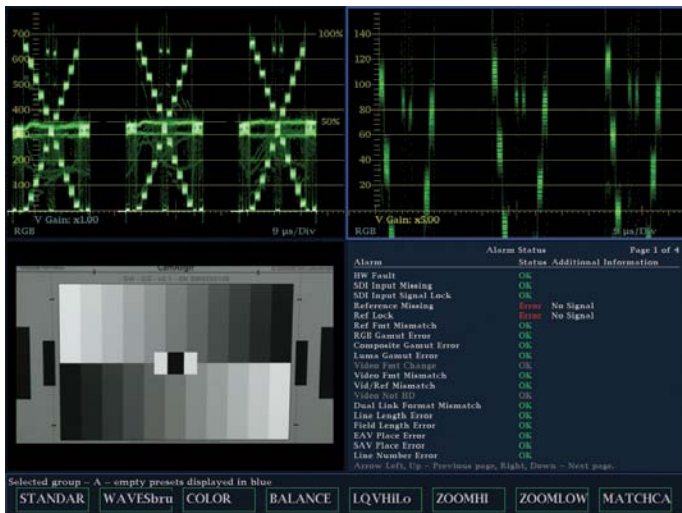
Figure 9. This shows a standard RGB Parade at the top left. On the top right the image is zoomed in and repositioned to show the detail of the highlights.
