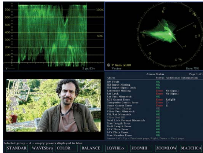
Figure 5. Note at the bottom of the screen that each preset has a customized name associated with a button. No need to scroll through menus to find a preset.
