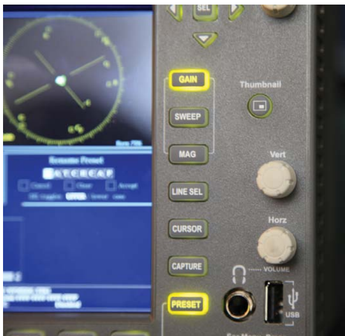
Figure 17. The front panel of the WFM5200 provides access to many dials and buttons that make it quick and easy to access the most important functions.
