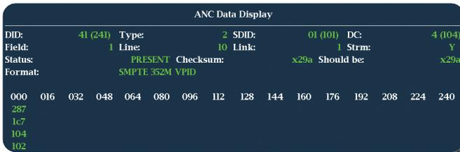
► **Figure 13.** *Ancillary Data Display of SMPTE 352M payload.*
