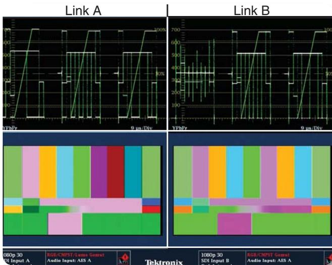
▶ **Figure 7.** Waveform displays of Dual Link A and B signals for R'G'B' 4:4:4 12-bit format.
