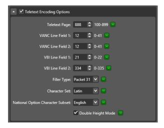
Naturally, the Teletext OP47 MXF output parameters include Teletext Encoding Options. These options allow you to configure the Teletext encoding settings. Please refer to your TV station's or video programming distributor's delivery requirements to select the appropriate Teletext settings.
