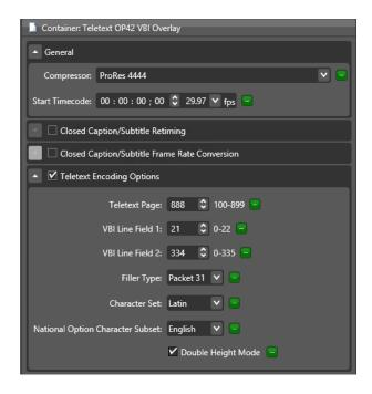
When setting up the Flip action to combine the OP-42 Teletext VBI graphics (.mov file) with video, a Movie Overlay filter must be applied to process the .mov file that is created with Timed Text Flip.
