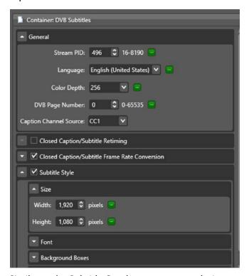
Similar to the Subtitle Overlay output, a resolution must be specified for the DVB Subtitles output. This resolution should be limited to the specifications of DVB Subtitling which include SD, 720, and 1080. In addition, DVB also requires you to specify the PID number, color depth, and language tag for each language in a Transport Stream.
