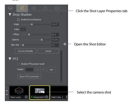
5. Click the PTZ triangle to display the PTZ controls. Check the Enable PTZ preset recall check box. Enter a preset number and click the Go arrow.
