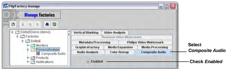
3. Click *Composite Audio* and select the *Decode Dolby E* option from the pull-down menu. This option causes the Composite Audio to decompose the Dolby E stream into up to eight channels of uncompressed audio:
