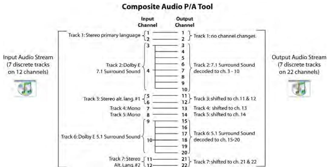
Notice that four of these channels are Dolby E encoded: one pair encoded as *7.1 Surround Sound*, the other as *5.1 Surround Sound*. These two pairs of Dolby E are decoded into a total of fourteen channels of uncompressed audio, whereas the remaining eight channels are passed through unmodified.
