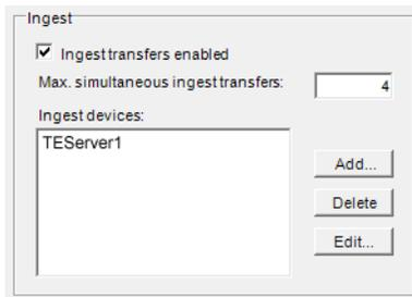
Enter/update the name of the Ingest Device. The Ingest Device name must match the name of the Transfer Engine server.
