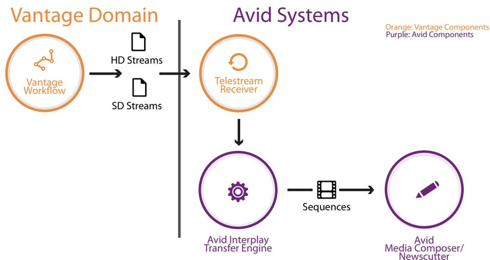
These components work together to enable Vantage workflows to automatically submit transcoded media to an Interplay Transfer Engine for background clip ingest, re-wrapping, and writing to an Avid editing storage volume (ISIS or DAS) for import into Media Composer and NewsCutter by operators.
