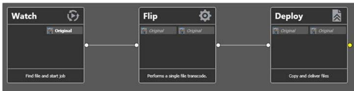
The basic workflow includes a Watch action to pick up new media, a Flip action with the Avid Transfer Manager/Transfer Engine Encoder configured to encode media per Avid requirements, and a Deploy action to deliver the encoded media to the proper location. When the workflow is activated, it polls a directory and—for each new file delivered—it starts a job to process the media through the workflow.
