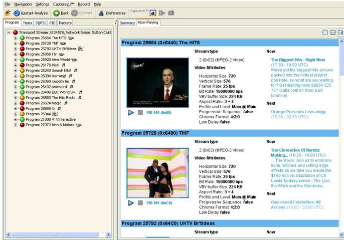
In addition to displaying a video thumbnail, the video format parameters from within ES headers are also displayed and can be checked for consistency with Transport Stream layer signaling of video parameters. This cross-check enables the operator to verify that the format of the content in the stream matches the format that they have signaled. An inconsistency could cause the STB to be unable to decode video and the viewers to lose their pictures.
