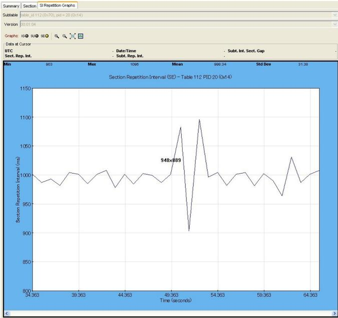
**Timing analysis** – The TSCA supports comprehensive PCR measurements to the TR 101 290 and A/78 standard. When the selected Elementary Stream PID contains PCR information, PCR trend analysis views are available, displaying graphs of: PCR accuracy, PCR arrival interval, PCR overall jitter, PCR frequency offset, and PCR drift rate.
