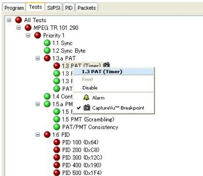
The captured stream can also be permanently stored on the hard disk for subsequent reanalysis with the deferred time TSCA application. This powerful debug mode enables fast debugging of troublesome intermittent problems. CaptureVu technology also supports triggering events based upon IP Layer measurements, providing integrated cross-layer fault analysis and logging in a single box solution for network fault diagnosis.
