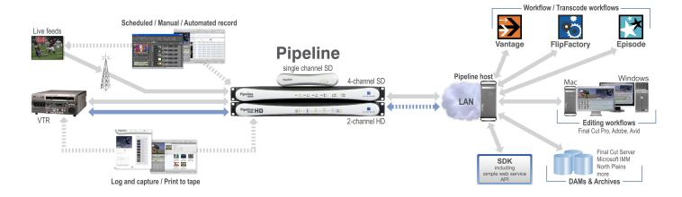
This standard definition SDI video capture & play-out device offers real-time, user selectable SDI encoding to multiple formats. Schedule live feeds; log & capture from tape; or ingest into any file-based workflow.
