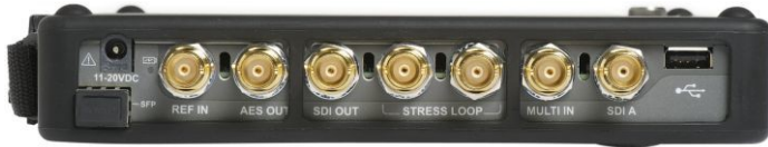
WFM2300 top panel connectors.
