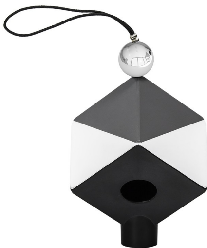
Reference object, Specular highlight, 90% white, 18% gray, black and light trap.
