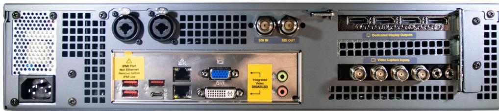
Gear model). If you have a 400 series, there will be an additional SDI Input connector and additional SDI output connector on the chassis itself, and not an EXT card.
