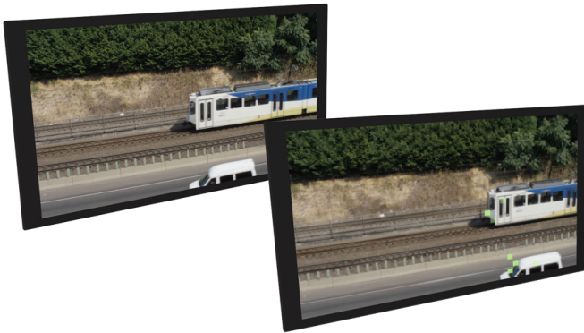
Figure 5: Misalignment across Video Output Streams
