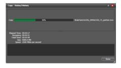
**Note:** Vantage will display throughput as Mbits/s and not Mbytes/s, so you will need to divide by 8 to get units which match benchmarking and copy results.
