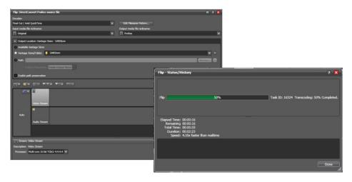
In the above test we are seeing  $\sim$  4.3x faster than real time conversion. Repeat the same test with 4 x Apple Pro Res source files submitted simultaneously and note performance. In our example each DirectConvert performed at 2.7x real time or an aggregate throughput of 10.8x real time.
