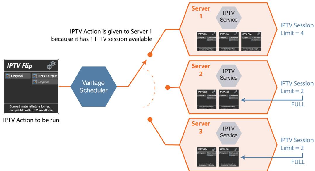
Session Based load balancing offers good, basic load balancing as a starting point for Vantage Array systems, and it comes built-in and operating with the Array license. You can make adjustments to this automatic system by setting the session limits for each service. If your Vantage system utilizes a combination of multiple transcoding services, then using Task Based load balancing will allow you to balance between these services providing optimal machine saturation.
