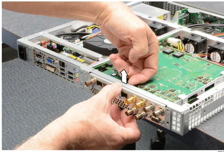
**Figure 27: Install the rear plate panel**
