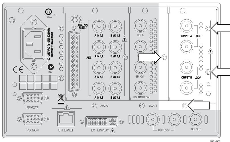
**Figure 8: Removing the Slot 2 rear-panel screws**
