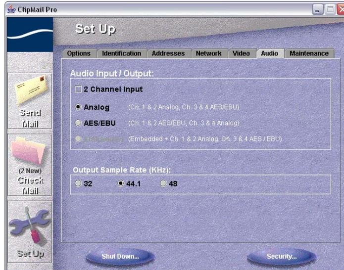
Check 2 Channel Input if you have 2 audio channels, then select either Analog, AES/EBU or Embedded (when SDI is selected for video).
