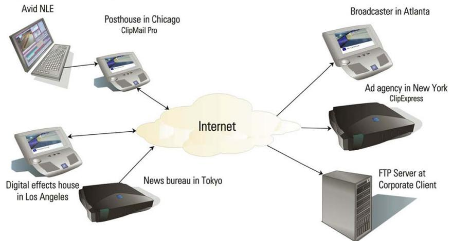
Using the Digital Cut feature on any Avid, ClipMail is treated like a VTR or any other RS-422 controllable device. Instead of printing to tape, you can create a digital file using ClipMail Slave Mode Encoding. Using ClipMail's Auto Send feature, ClipMail can automatically deliver the file to any number of recipients, anywhere in the world via the Internet.
