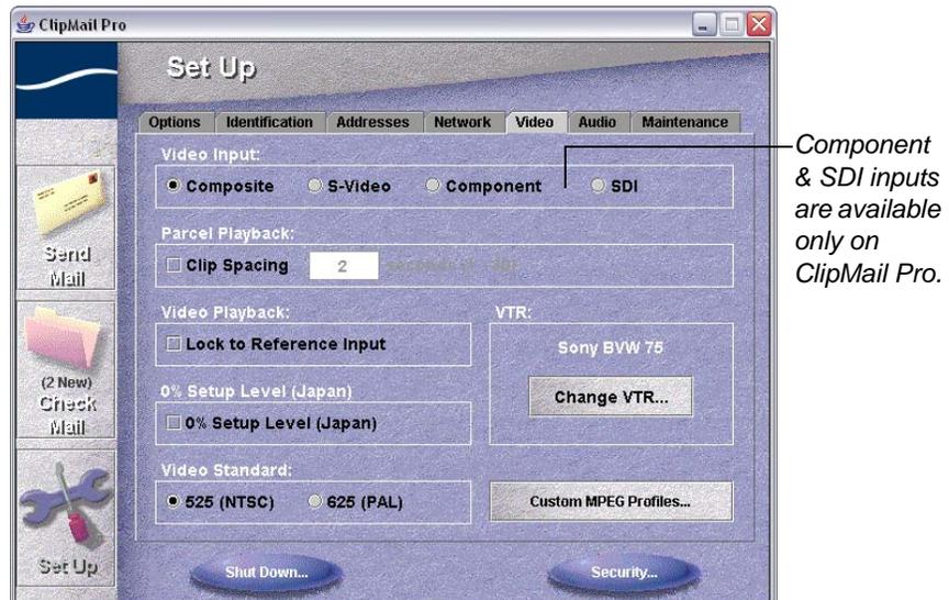
The Video and Audio menu panels allow you to select your audio and video inputs from the available connectors on the rear panel of the appliance, and configure settings for each.
