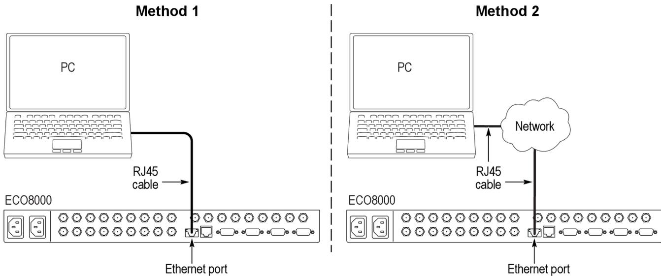
Figure 11: Equipment connections for Test 16
