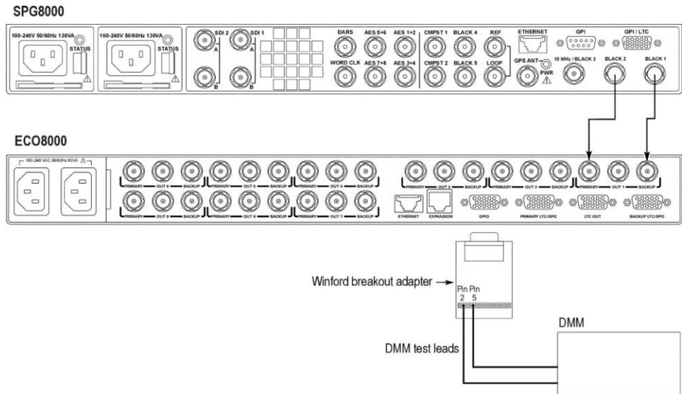
**Figure 8: Initial equipment connections for Test 13**
