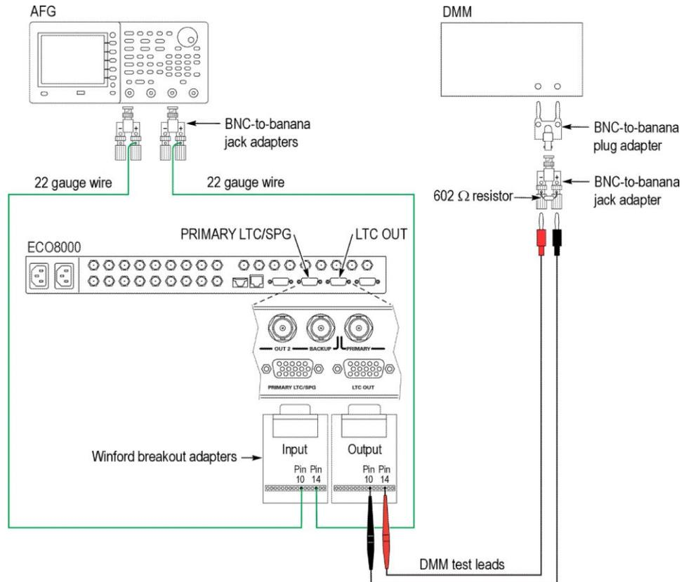
**Figure 6: Equipment connections to test LTC 1 for Test 11**
