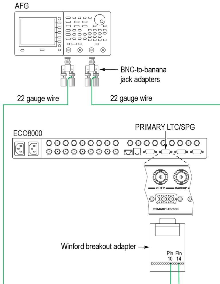
**Figure 7: Initial equipment connections for Test 12**
