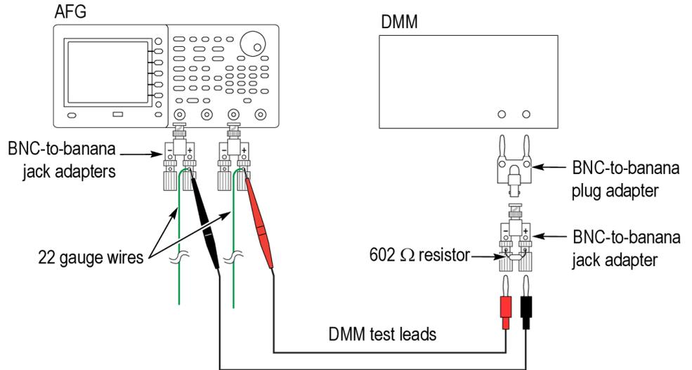
**Figure 5: Equipment connections to characterize the AFG output for Test 11**
