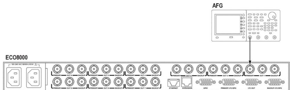
**Figure 4: Initial equipment connection for Test 10 (ECO8000 shown)**
