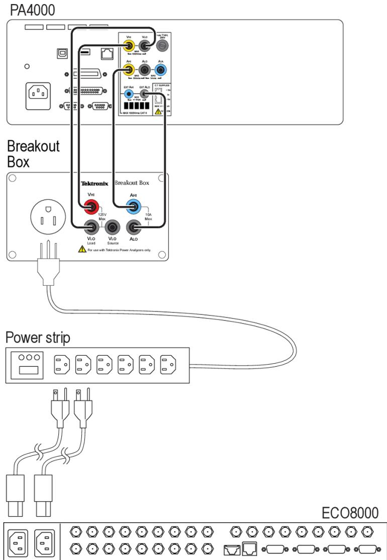
**Figure 1: Equipment connections for Test 4 (ECO8000 shown)**
