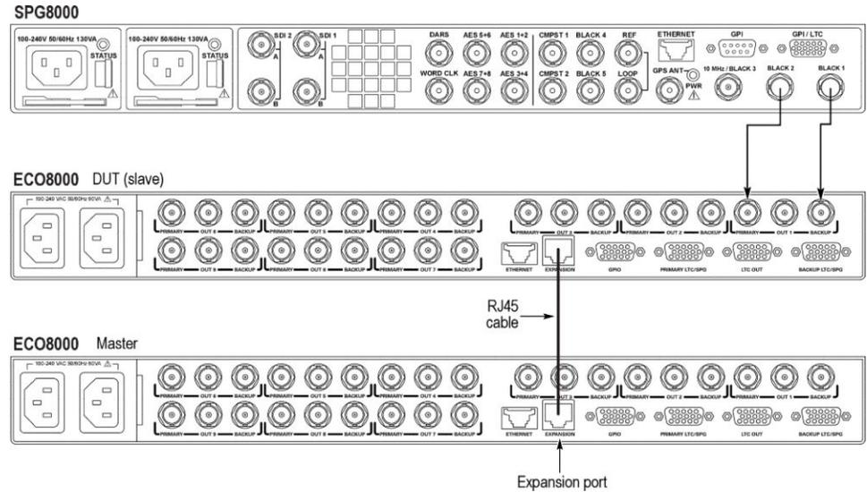
Figure 10: Initial equipment connections for Test 15
