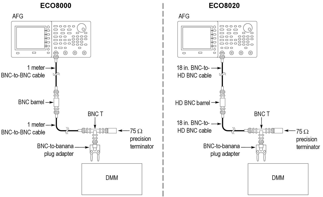
**Figure 3: Initial equipment connections for Tests 8 and 9**
