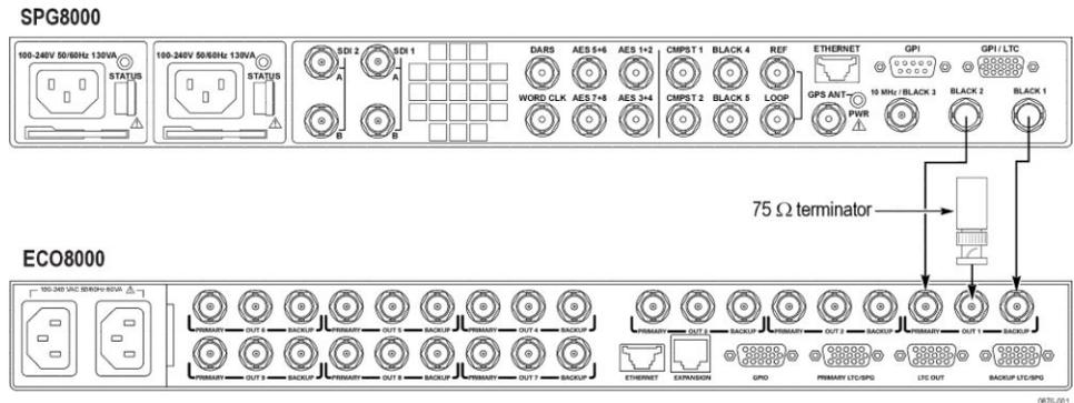
**Figure 2: Equipment connections for Test 7 (ECO8000 shown)**
