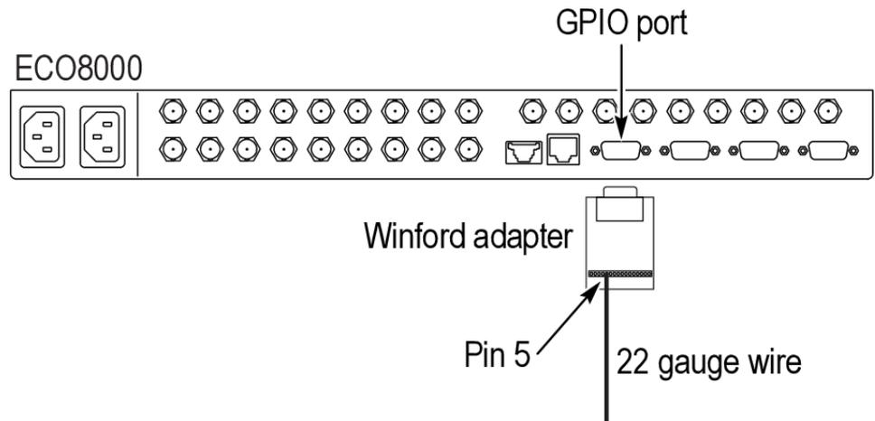
**Figure 9: Initial equipment connections for Test 14**
