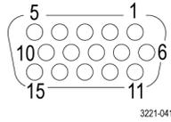
**GPIO connector signal pinouts**
