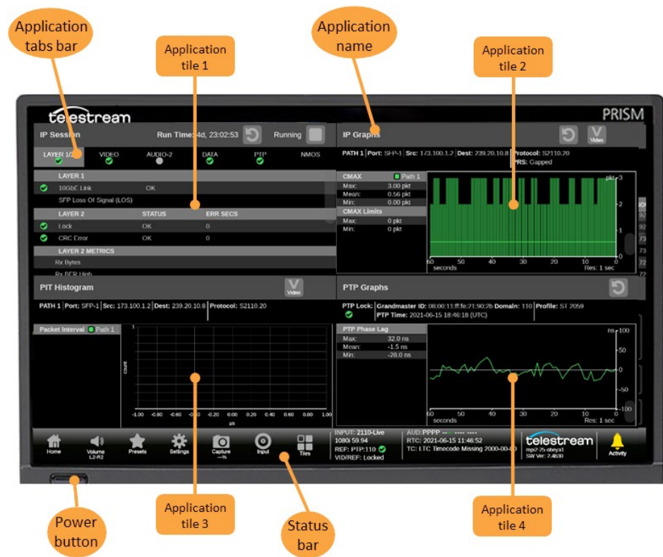
Figure 6: Elements of the front panel
