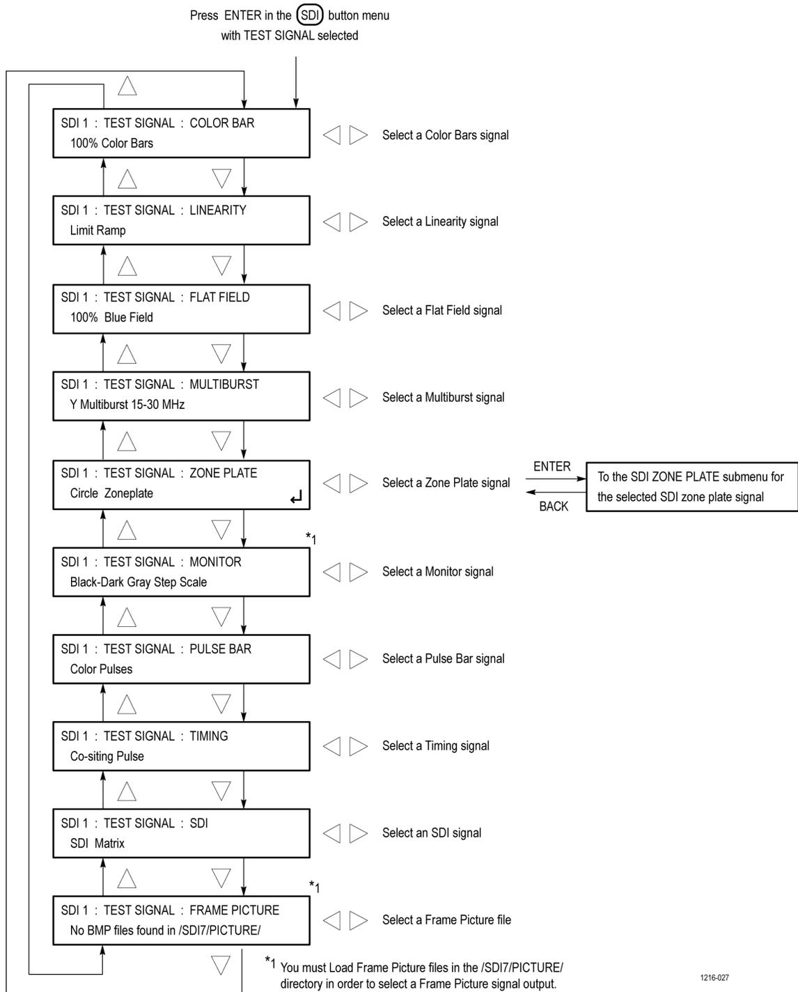
**Figure 85: SDI TEST SIGNAL submenu diagram**
