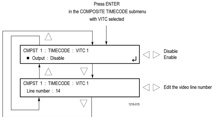
Figure 72: COMPOSITE TIMECODE VITC submenu diagram
