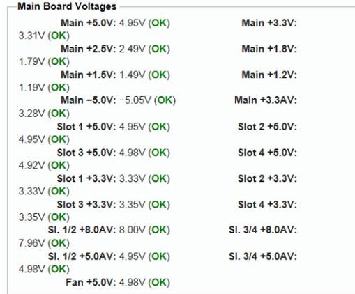
**Figure 48: Main Board Voltages diagnostic readouts**
