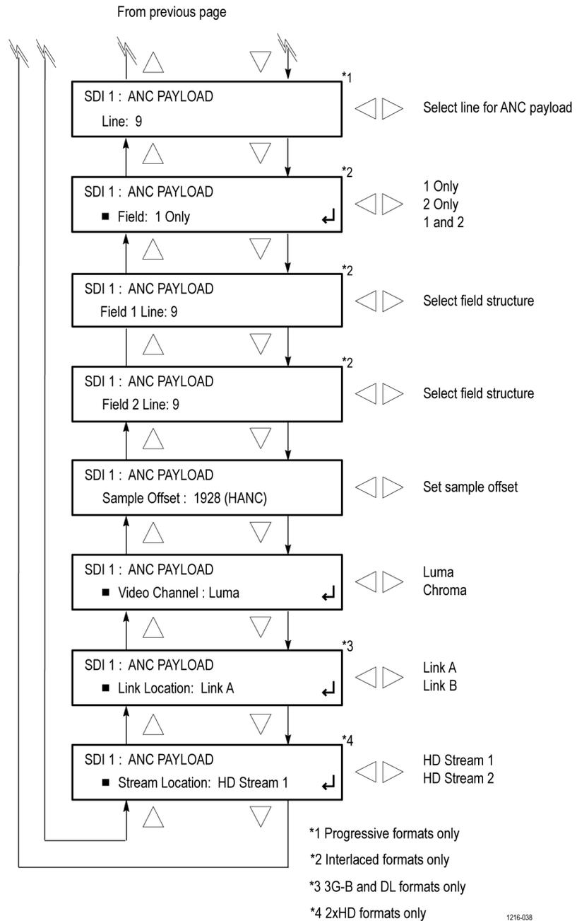
Figure 96: SDI ANC PAYLOAD submenu diagram – part 2
