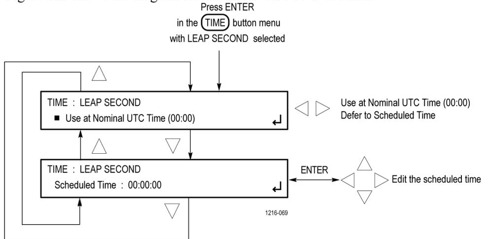
**Figure 122: LEAP SECOND submenu diagram**
