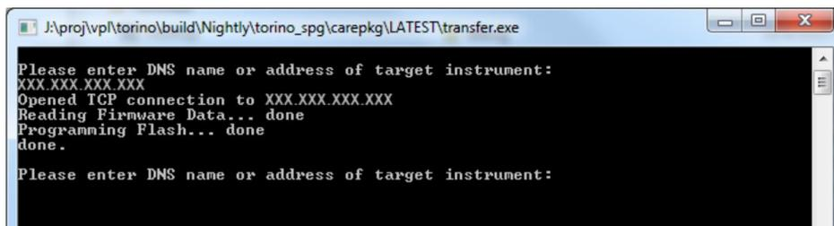
Figure 6: Sample of transfer.exe window after the upgrade is complete
