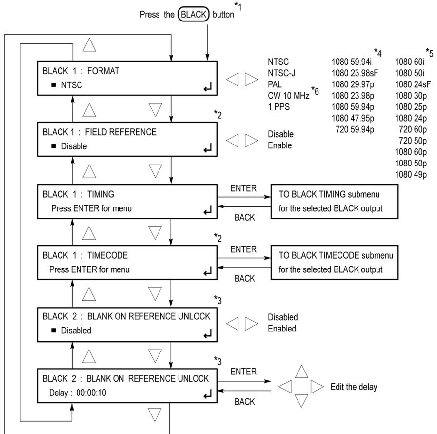
\*1 Press the **(BLACK)** button repeatedly to select the desired BLACK output (1-5) or to select the desired group of Black outputs (1-3 or 4-5). BLACK outputs 1-3 are standard; BLACK outputs 4-5 are available with Option BG only. When you select a group of BLACK outputs, you can set whether a non-integer or an integer clock will be used for the HD tri-level sync rate for those outputs.
