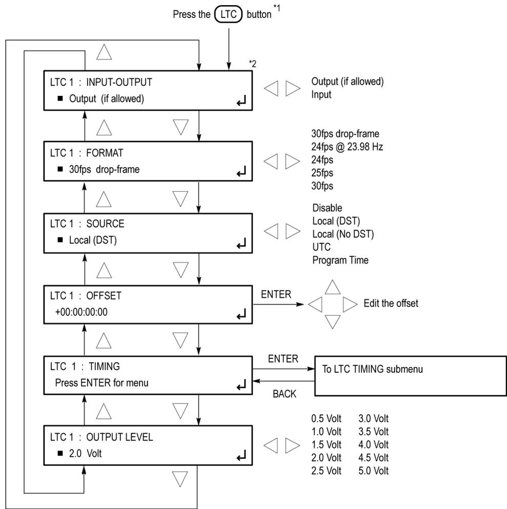
\*1 Press the **LTC** button repeatedly to select the desired LTC signal (1-4).
