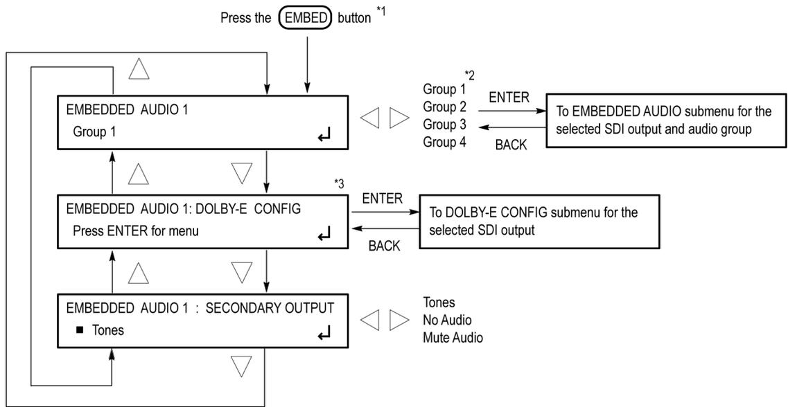
\*1 Press the EMBED button repeatedly to select the embedded audio for the desired SDI output (1 or 2).
