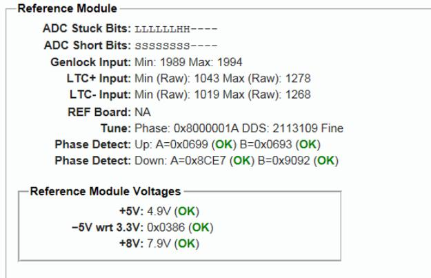
**Figure 49: Reference Module diagnostic readouts**
