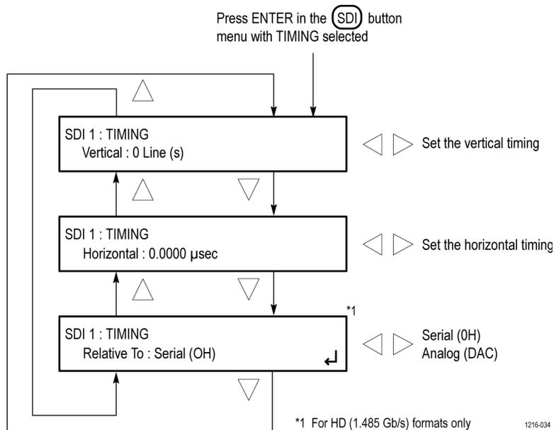
Figure 92: SDI TIMING submenu diagram
