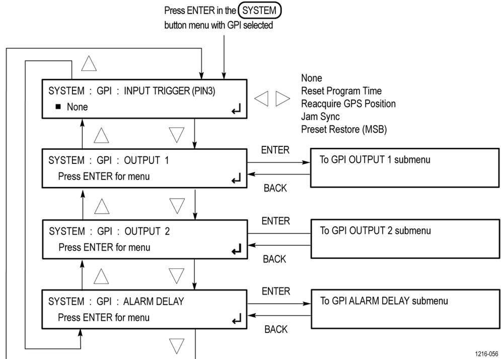
Figure 108: GPI submenu diagram
