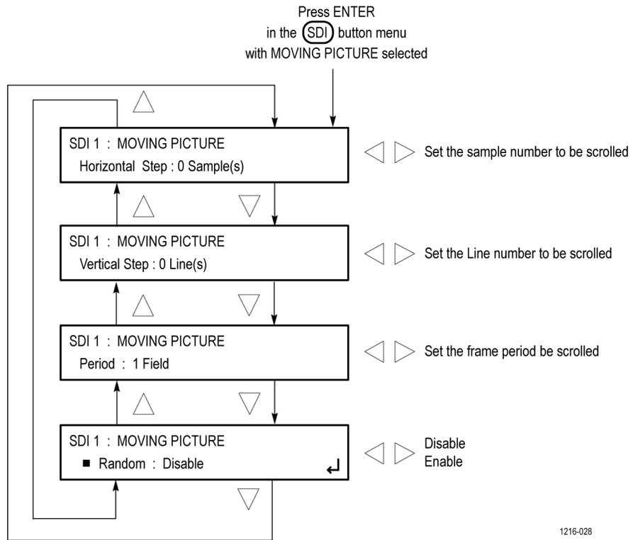
**Figure 86: SDI MOVING PICTURE submenu diagram**
