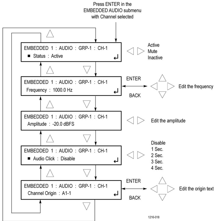
Figure 75: EMBEDDED CHANNEL submenu diagram
