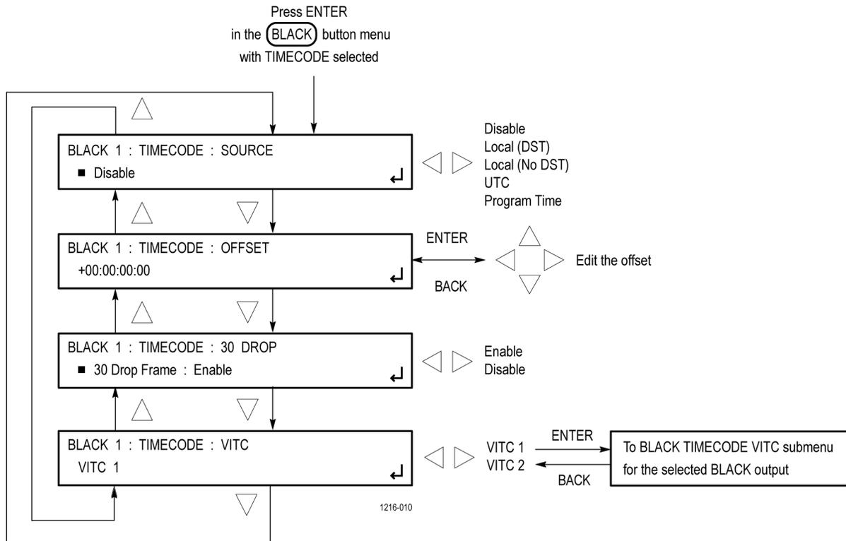
Figure 67: BLACK TIMECODE submenu diagram
