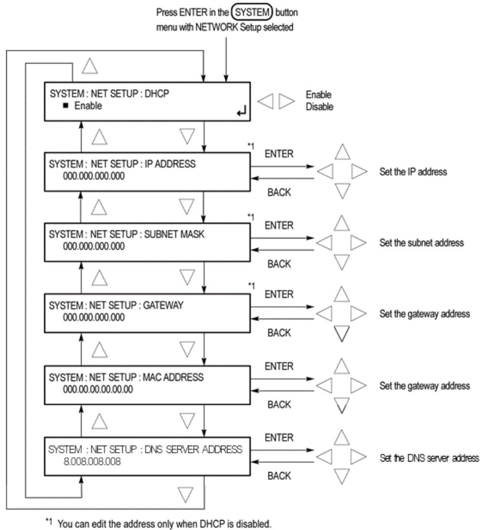
Figure 103: NET SETUP submenu
