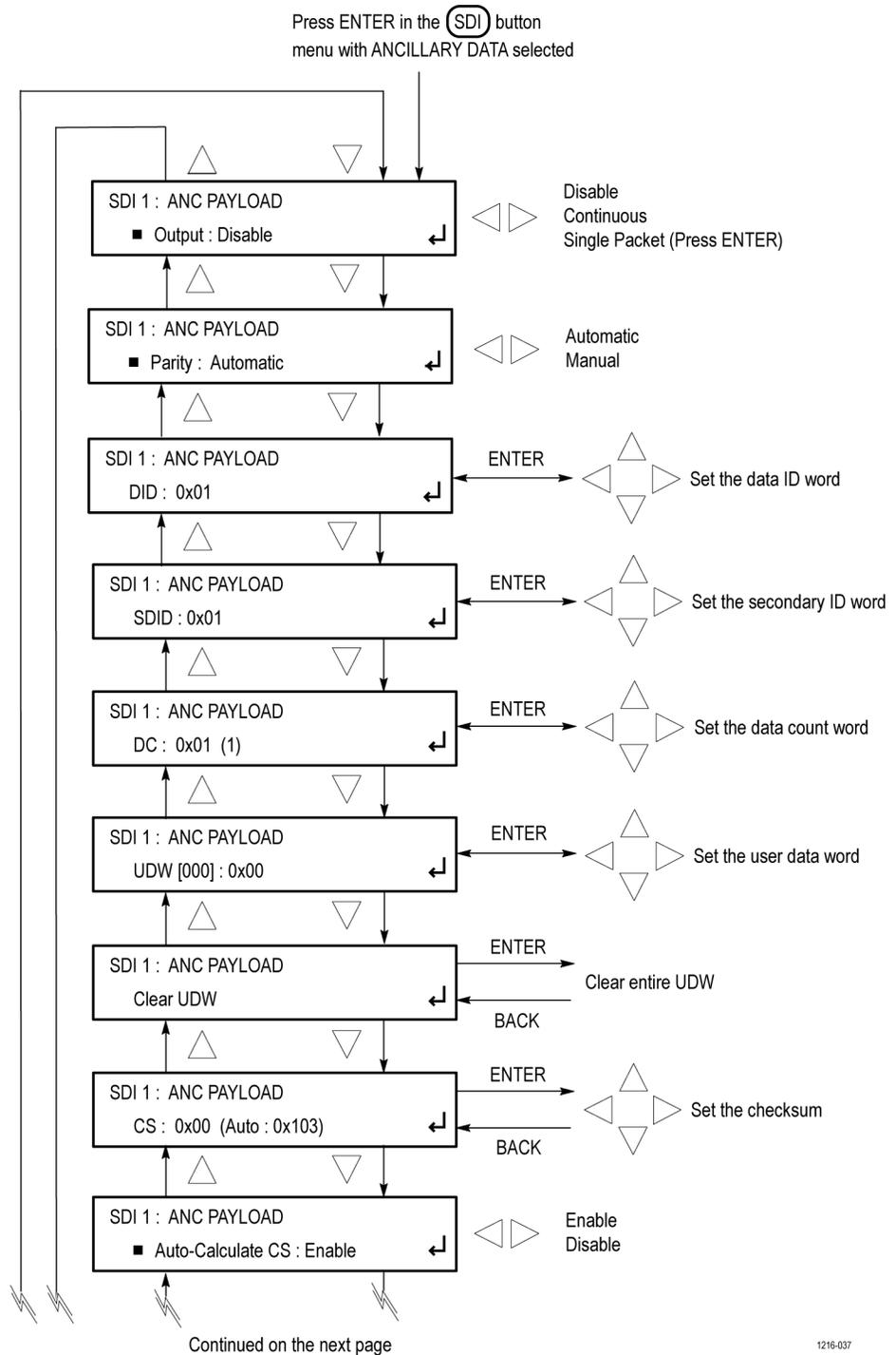
**Figure 95: SDI ANC PAYLOAD submenu diagram – part 1**
