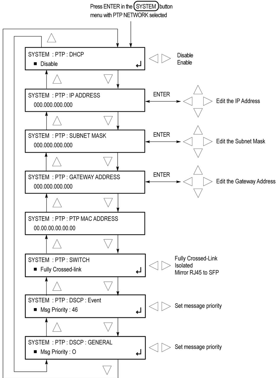
SYSTEM button - PTP NETWORK submenu diagram
