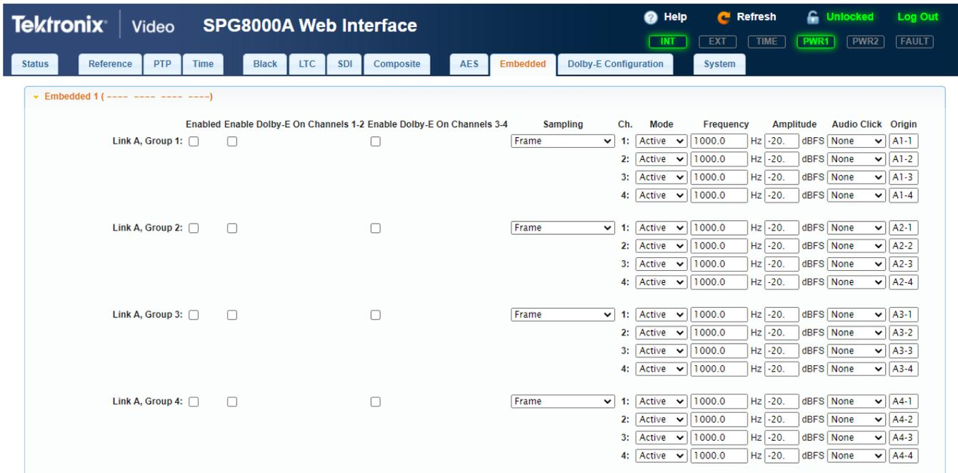
Figure 12: Partial Embedded menu diagram
