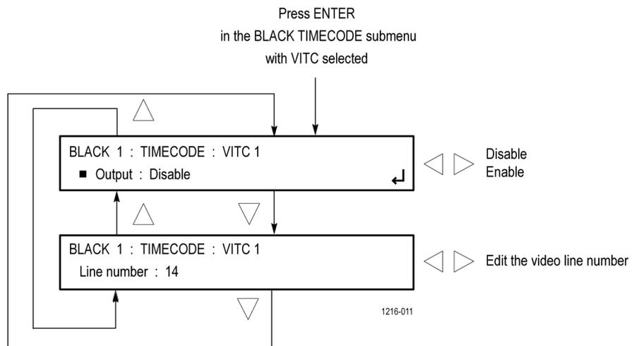
Figure 68: BLACK TIMECODE VITC submenu diagram
