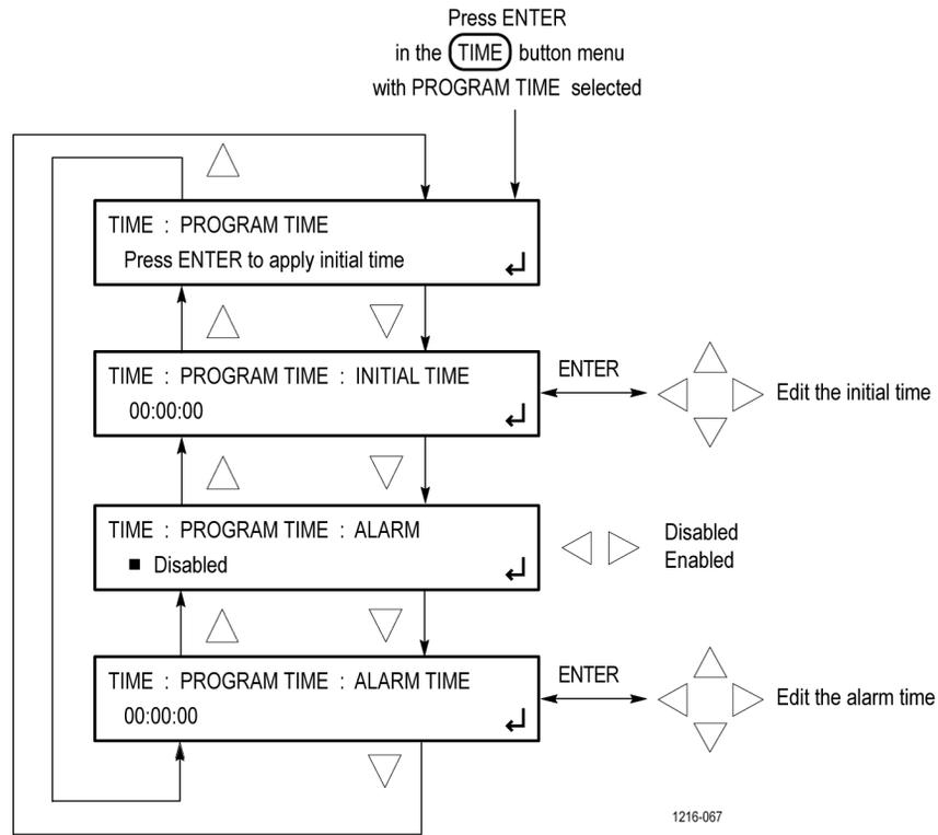
**Figure 120: PROGRAM TIME submenu diagram**
