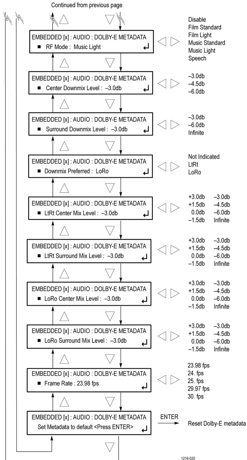
Figure 77: DOLBY-E CONFIG submenu diagram – part 2
