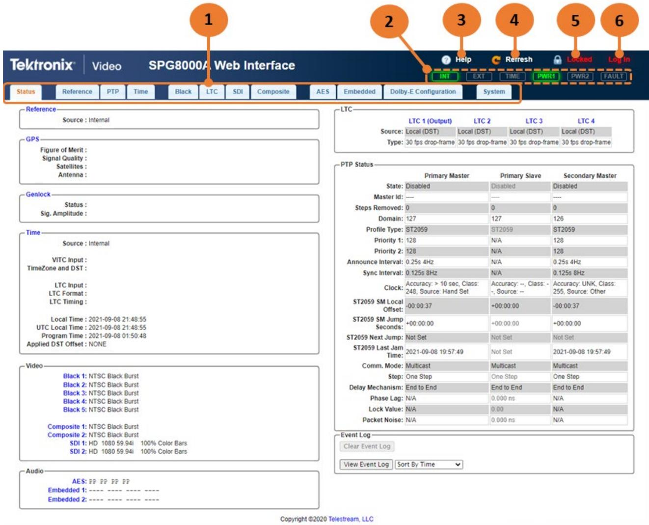
Figure 2: Example SPG8000A web user interface window
