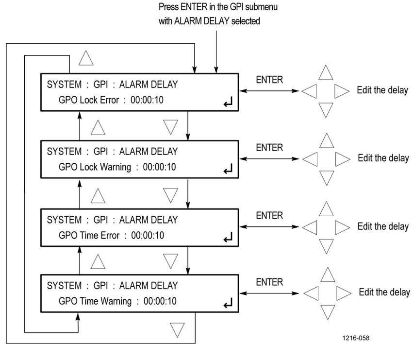
**Figure 110: GPI ALARM DELAY submenu diagram**
