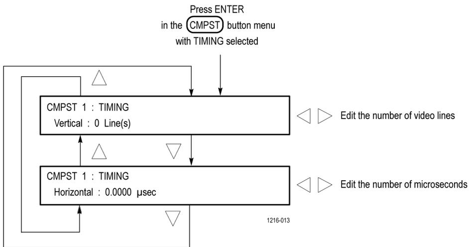
**Figure 70: COMPOSITE TIMING submenu diagram**
