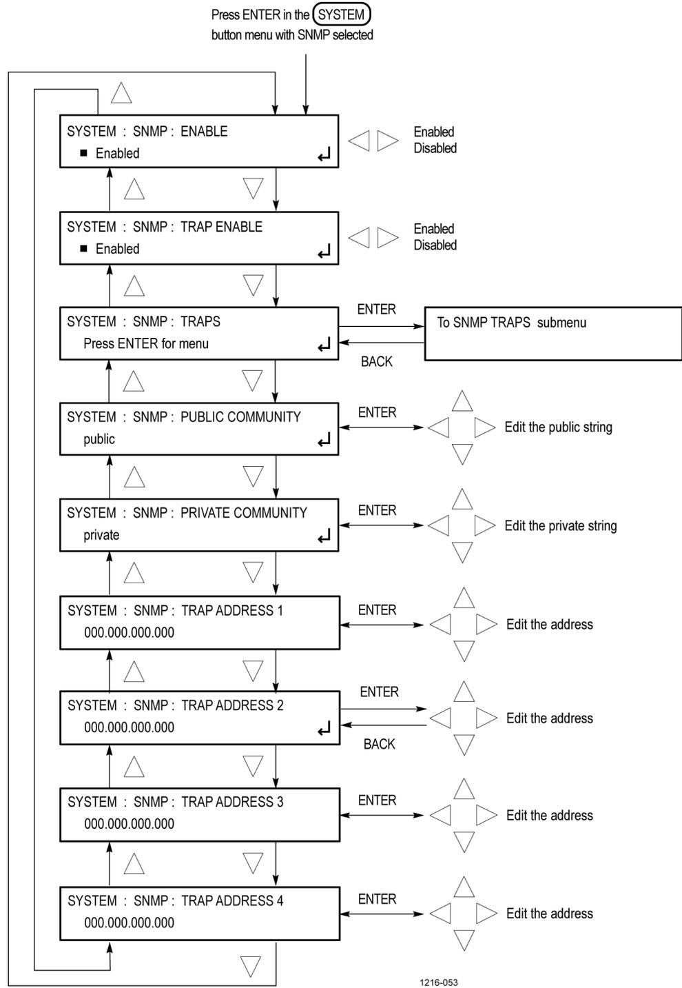
**Figure 105: SNMP submenu diagram**
