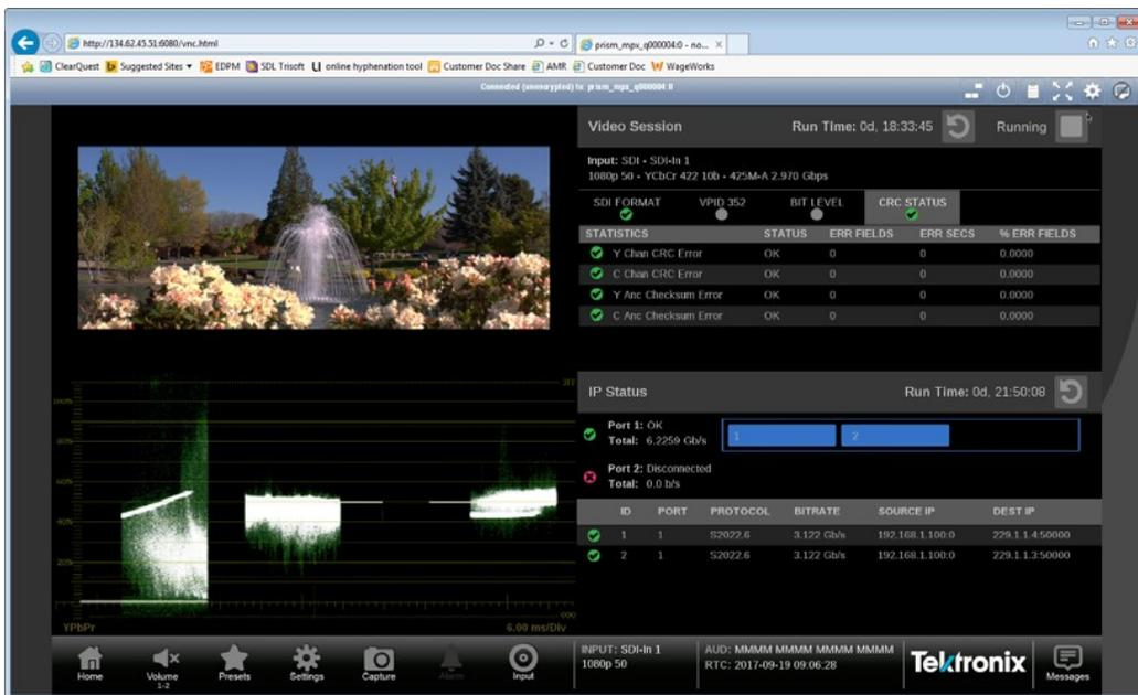
7. The web browser connects to the instrument with the browser display appearing exactly like the display on the external monitor, but with a slower update.
