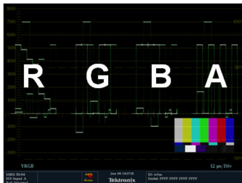
Figure 14: Dual Link information placement in waveform display
