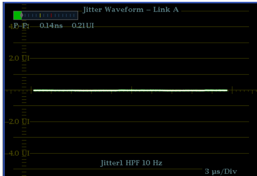
Figure 36: The Jitter display parameters as shown in a single tile when the instrument is in 4-tile mode
