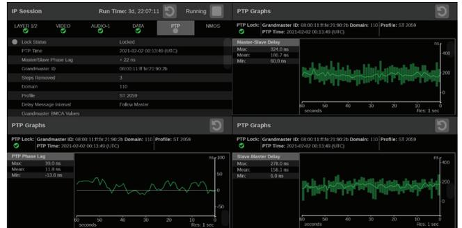
FIGURE 21. Monitoring PTP performance with PTP Graphs displays.
