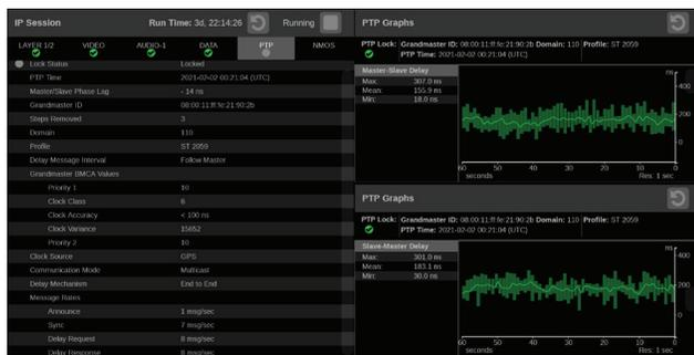
FIGURE 21. Monitoring PTP using PRISM's IP Session and PTP Graphs displays.
