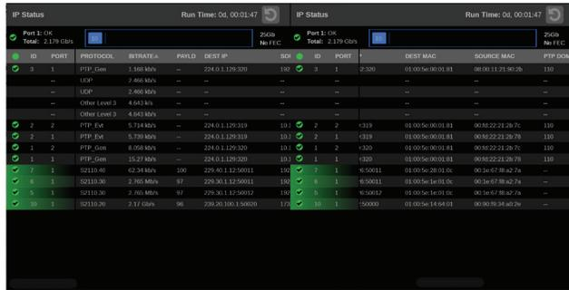
FIGURE 20. PRISM IP Status showing IP streams on the ports and PTP traffic with domains present.
