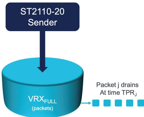
FIGURE 5. Virtual Receiver Model
