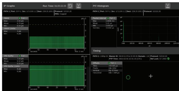
FIGURE 15. Prism CMAX and VRXFULL measurements for ST2110-20.
