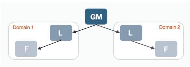
FIGURE 18. PTP Domains Synchronized to a Common Grandmaster
