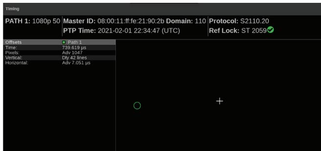
FIGURE 14. Prism Timing Display show PTP lock to a 3G 1080p50 signal.
