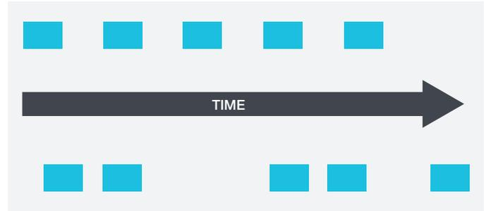
FIGURE 1. Packet jitter is deviation from the periodicity of the packet arrival interval.
