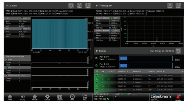
FIGURE 27. IP Graphs and PIT Histogram of Prism showing IP stream information.
