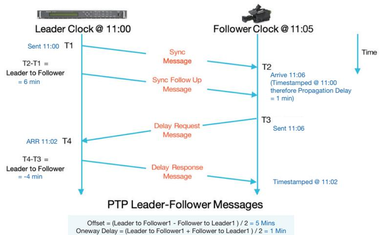
FIGURE 19. Deriving the Correct Time in a PTP Network.
