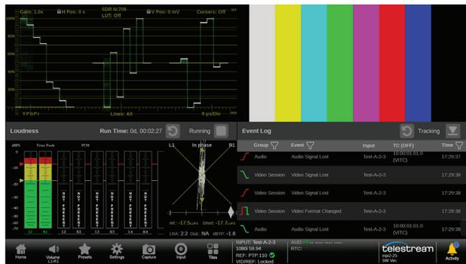
FIGURE 25. Prism decoding an IP stream showing waveform, picture, audio bars and event log.
