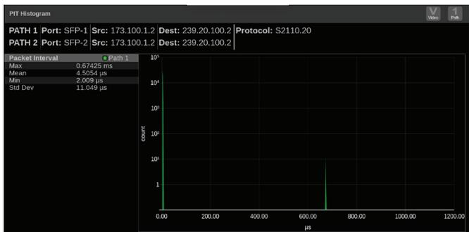
FIGURE 10. Histogram of ST2110-20 Narrow Gapped Sender.
