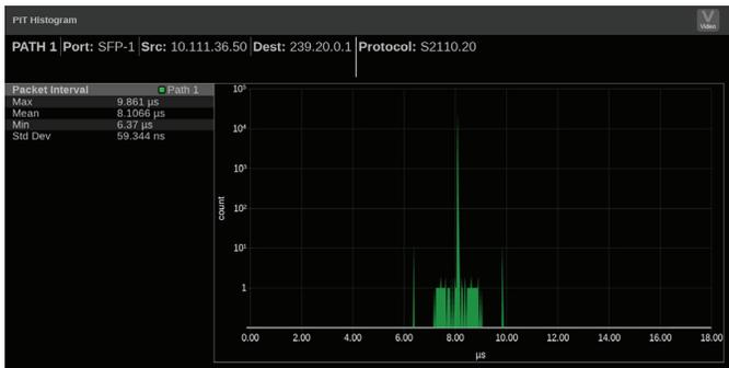
FIGURE 9. Histogram of ST2110-20 Narrow Linear Sender.
