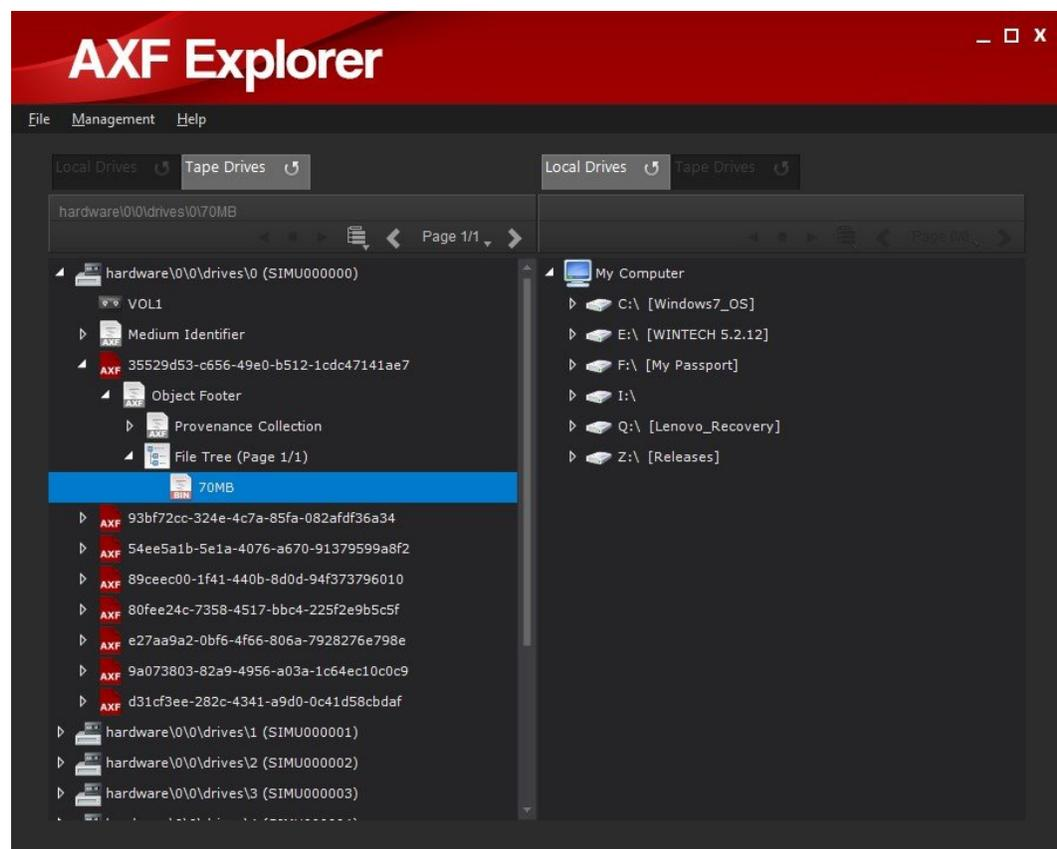
The number of file components displayed within the file navigation tree of an AXF object is set to a fixed value per page. You modify this setting on the Configuration screen. Each page will only display a subset of files, keeping the file navigation tree easy to read.
