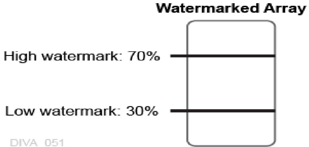
The following figure represents a watermarked disk array with permanently stored objects with a total size that is less than the Low Watermark:
