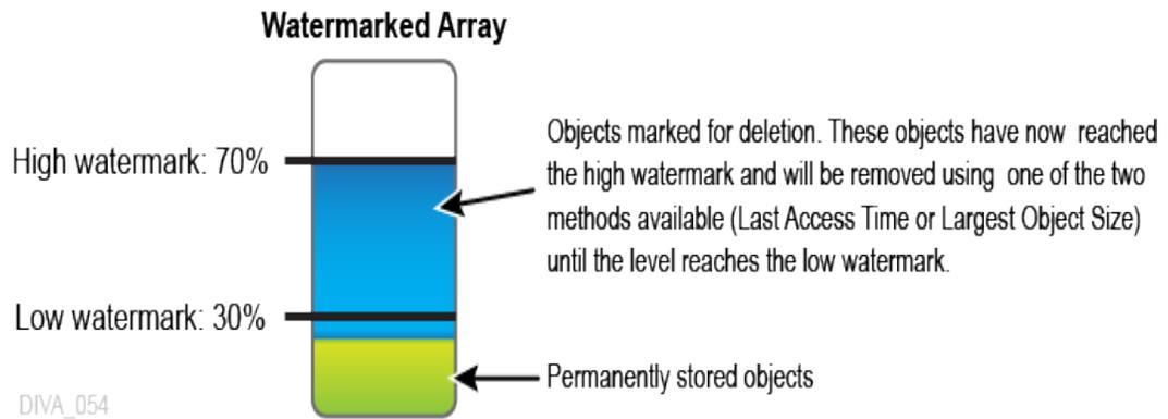
The following figure represents a watermarked disk array after the temporary objects have been deleted down to the Low Watermark. Objects have now been deleted (*either by Last Access Time or Largest Object Size*) and the Low Watermark has been reached. At this point, object deletion stops until the High Watermark is reached again; then the process repeats.
