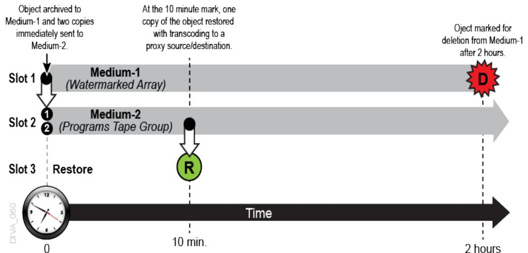
The following figure is an example of a SPM configuration with one copy left in the online tape group (Medium-2 named Programs), and a second backup copy made to a different tape group (Medium-3 named Backups) that is to be taken offline. In this example, one copy is kept on the SPM watermarked array (*with Watermark set to Yes*) for two hours, and two copies are made immediately. One copy is made to a tape group named Programs, the second copy is made to a different tape group named Backups.
