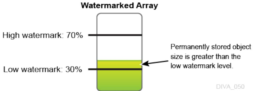
The following figures characterize a typical Watermarked Medium (watermarking set to Yes) and illustrate how watermarking ensures the medium does not reach full capacity.
