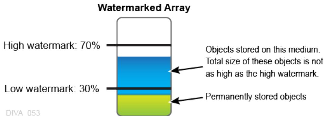
The following figure represents a watermarked disk array with permanently stored objects with a total size that is less than the Low Watermark, and temporarily stored objects with a total size that has reached the High Watermark level. In this figure the temporary objects have now reached the High Watermark, and will be removed using one of the two methods available (*Last Access Time* or *Largest Object Size*) until the level reaches the Low Watermark.
