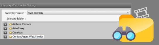
ContentAgent can detect master clips or sequences dropped into an Interplay folder and initiate an automated workflow.
