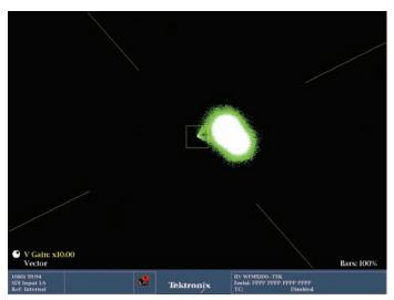
Figure 4. Vector display with incorrectly adjusted output from the camera.
