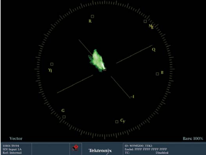
Figure 7. Vectorscope of the warmer piano shot. Notice that the trace leans towards the red vector.
