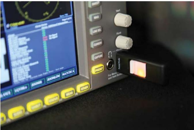
Figure 22. After properly dismantling the "thumb drive" from your computer, plug it in to the USB port on the front of the WFM5200 or other Tektronix waveform monitor.
