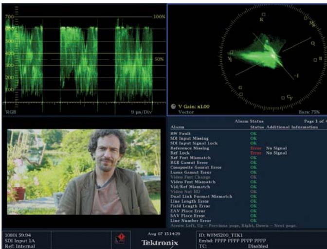
Figure 3. WFM 5200 Option CAM with 4 different inputs.
