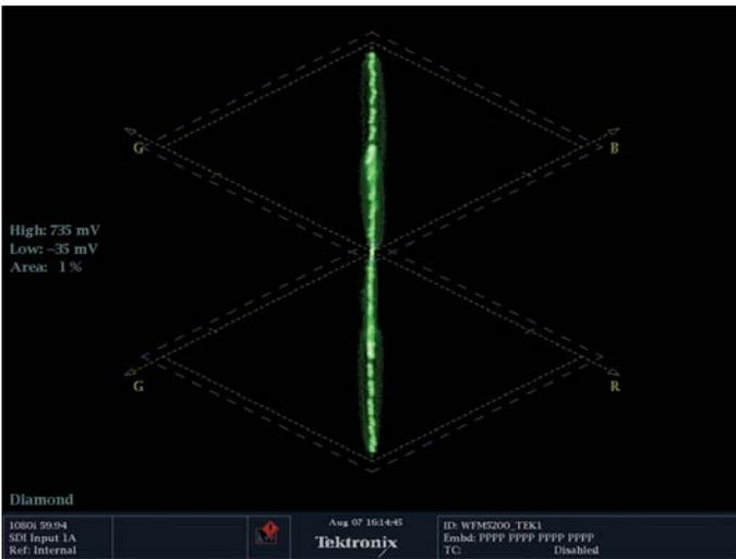
Figure 13. With the line running vertically up the middle, the image is balanced.
