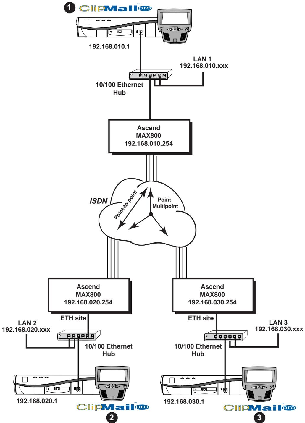
Figure 1. Example of an Ascend MAX800 System Configuration
