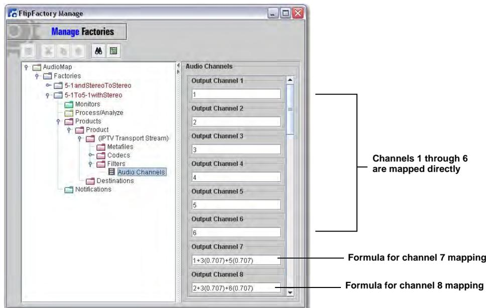
This example uses the *IPTV Transport Stream* product and the codec is *iptv Stream*. This product defines the 5.1 channels differently than the input 5.1 audio source: left (1), right (2), center (3), left surround (4), right surround (5), low frequency (6). Notice that the low frequency channel is last in
