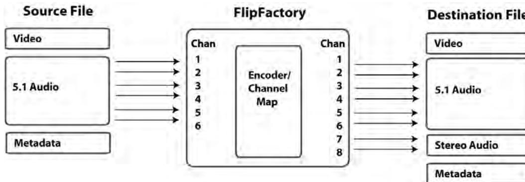
The first six channels of audio input represent the six channels of 5.1 audio: left (1), right (2), center (3), low frequency (4), left surround (5), right surround (6). Thus the mapping of audio input to output is direct. However, in order to down-mix the 5.1 audio to channels 7 and 8, down-mix formulas are entered for output channels 7 and 8.
