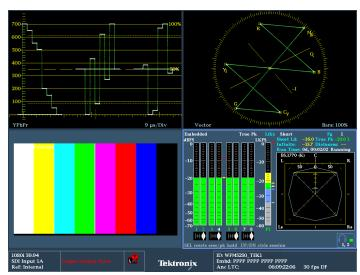
Quad Tile display allows for displays to be viewed simultaneously.
