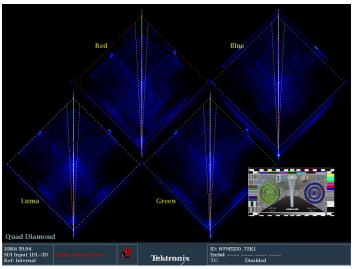
Quad Diamond display for stereoscopic alignment.
