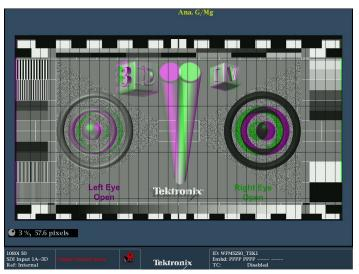
3D monitoring using a disparity grid.
