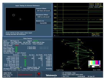
Timing and Lightning displays simplify timing tasks.
