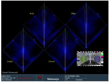
Quad Diamond display for stereoscopic alignment.
