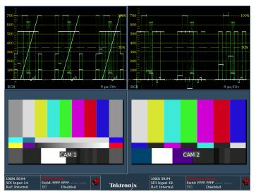
Two-channel simultaneous monitoring of waveform and picture input, ideal for monitoring multiple camera inputs.
