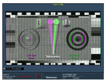
3D monitoring using a disparity grid.
