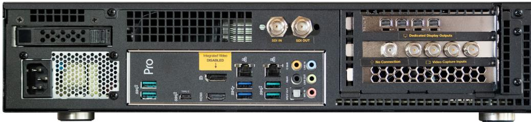
3. **Connect displays:** connect one or more displays via DisplayPort. This is accomplished either directly via Mini DisplayPort connectors, or via DisplayPort using the included Mini DisplayPort to DisplayPort adapters.
