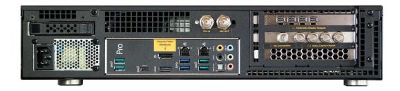
Connect displays: connect one or more displays via DisplayPort. This is accomplished either directly via Mini DisplayPort connectors, or via DisplayPort using the included Mini DisplayPort to DisplayPort adapters.
