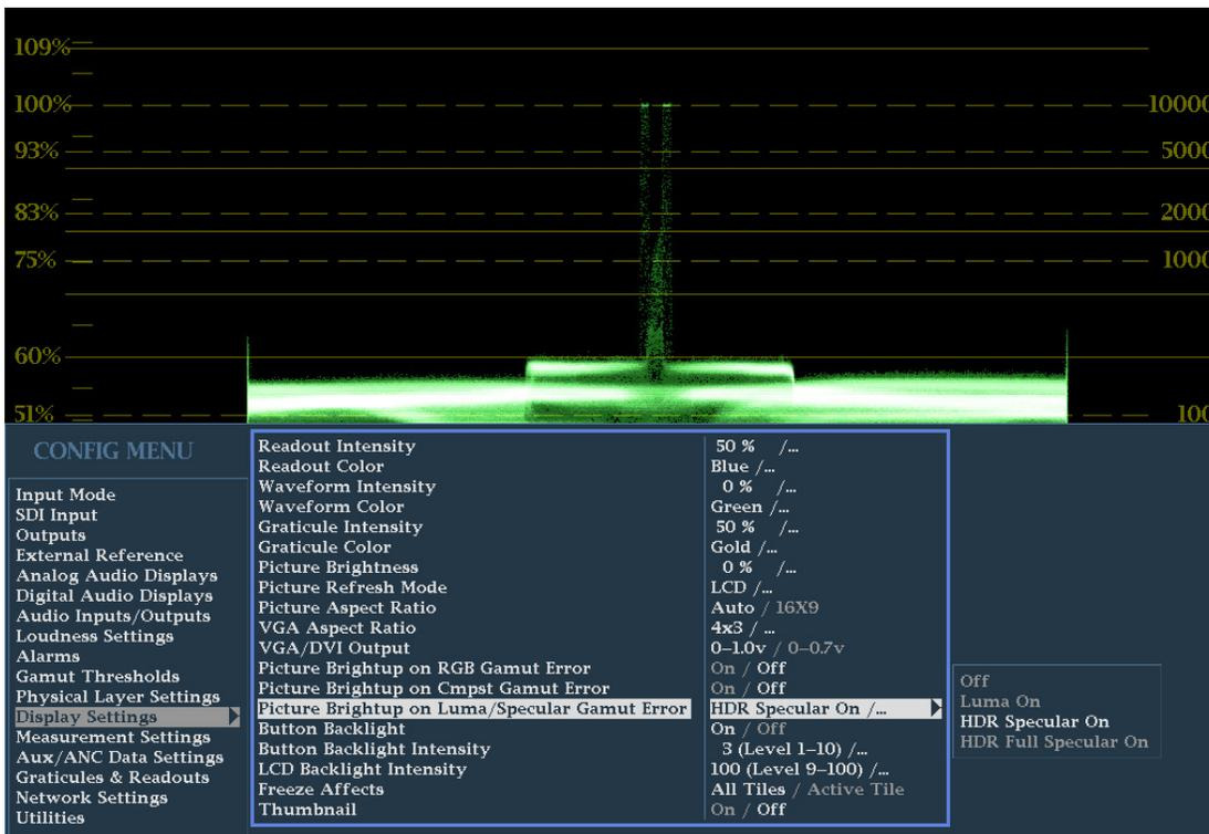
Figure 4: CONFIG menu showing the Picture Brightup on Luma/Specular Gamut Error selection
