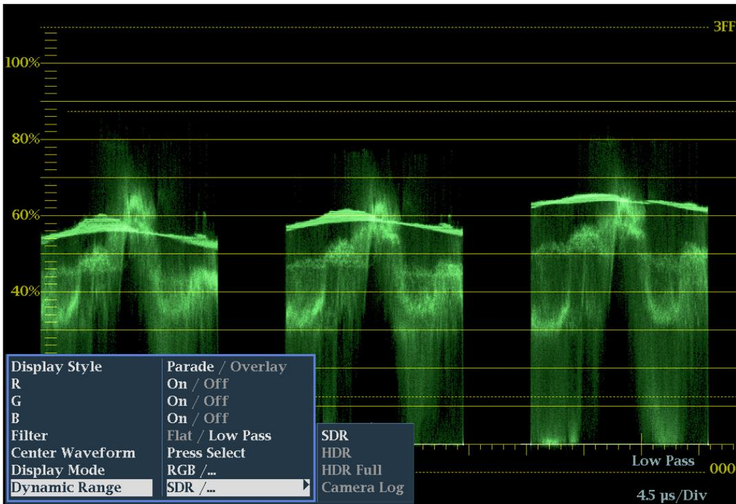
Figure 1: Waveform display pop-up menu showing the Dynamic Range selection
