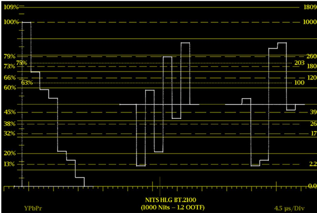
Figure 3: Waveform display showing the HDR graticule with NITS selected as the vertical scale
