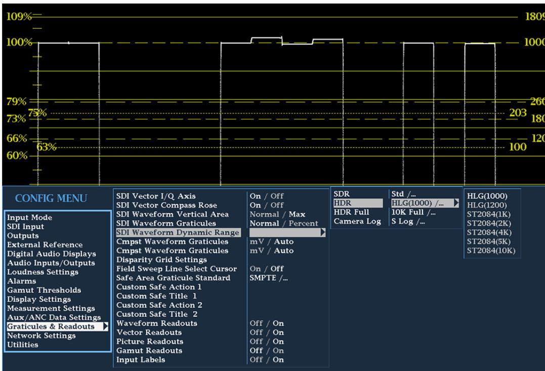
Figure 2: CONFIG menu showing the SDI HDR Waveform Graticule selection
