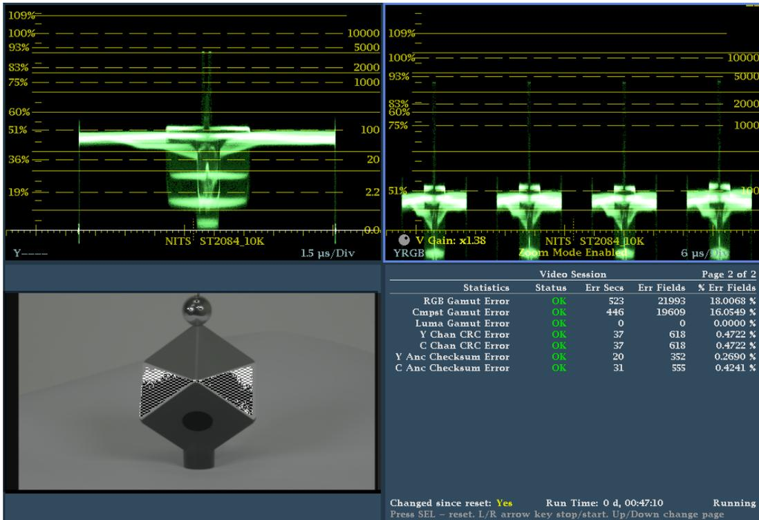
Figure 5: Typical HDR monitoring setup for ST2084(10K)
