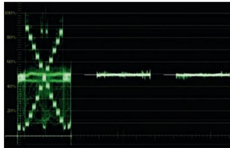
Figure 3-61 YCbCr Parade display of the chip chart in Figure 3-59.
