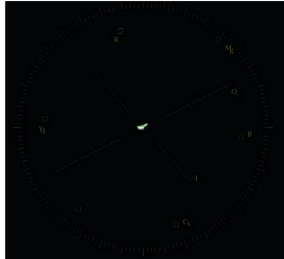
Figure 3-16 Vectorscope of white balanced paper at 90IRE.
