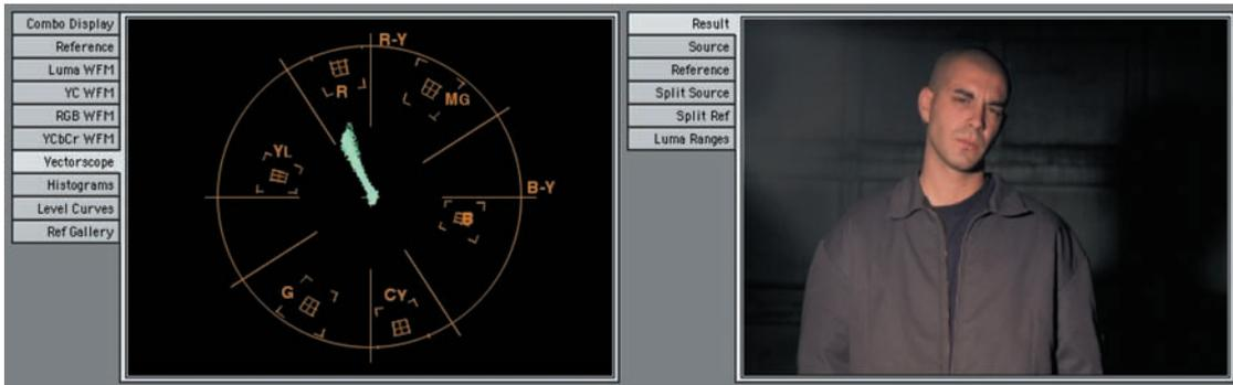
Figure 3-80 Screen capture from Synthetic Aperture's Color Finesse running in FCP. The video image is from Artbeats' Mixed Cuts Collection, shot LM113.
