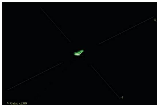
**Figure 3-68** Vector display of a white signal on a Tektronix WFM7120. The display has been zoomed in to magnify the center of the vectorscope 2x. This helps to center the white dot more accurately in the center of the vectorscope, assuring proper white balance.
