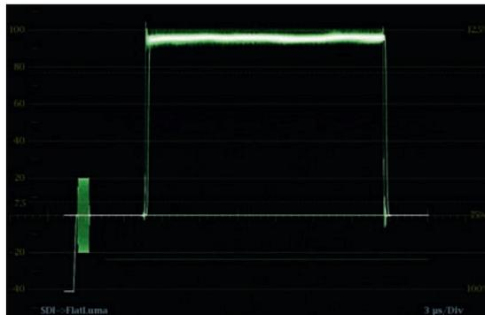
Figure 3-26 Flat Pass waveform display with very little excursion, showing that there is very little chroma, which means the whites are balanced. Compare this to Figure 3-20 from before the correction.
